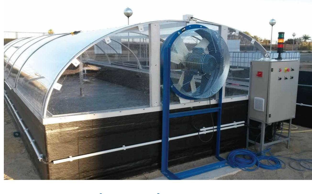
Evaporative technology designed taking into account minimal air volume contained within the greenhouse, control of the brine depth, control of temperature and humidity, thermal isolation of the ponds and considering air flow speed over the evaporation film.
