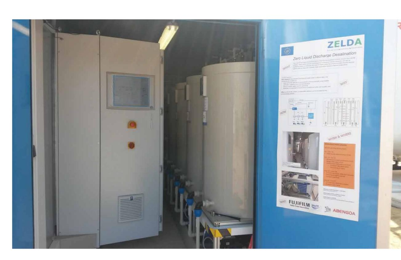
Electrodialysis metathesis (EDM) is an innovative electroseparation technology that allows the recuperation of two concentrates with high soluble salts. The EDM pilot plant consist of an ED stack with electrical and hydraulic connections, a control box, tanks with pumps, filling and drain piping and flow and pressure measurement units.
