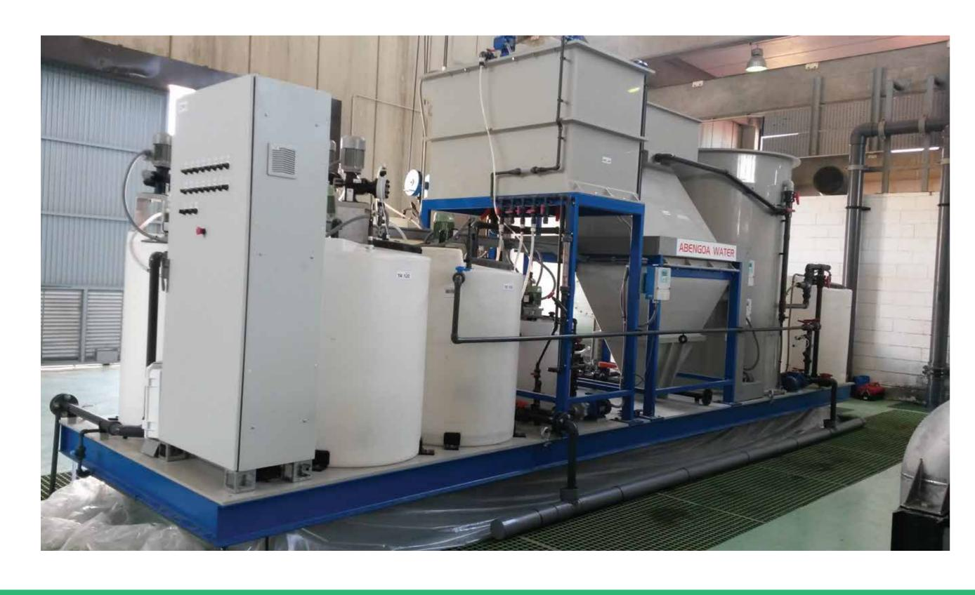
Pilot plant designed to purify high saline effluents.
