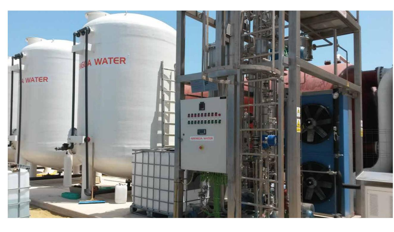
The pilot plant can operate under falling film or forced circulation and under different vacuum levels.
